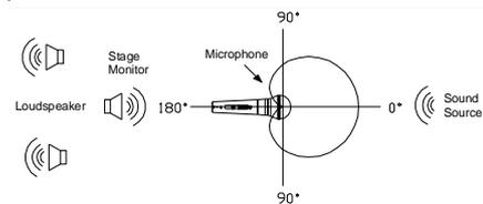
2. Do not cover any part of the grille with your hand, covering the grille alters the sound and distorts the polar pattern increasing the chance for feedback.
